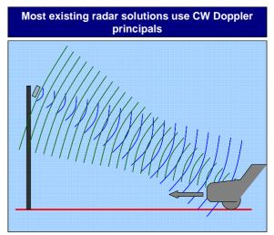
However if a target is static (i.e. not moving), there is no Doppler frequency shift in the returned echo, so the target is not registered. This is a serious limitation where the detection of static
