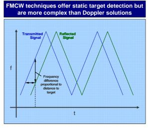
target distance can be deduced by comparing the transmitted frequency and echo frequency at any given time, and this is much easier to do than trying to measure the actual time delay directly.
